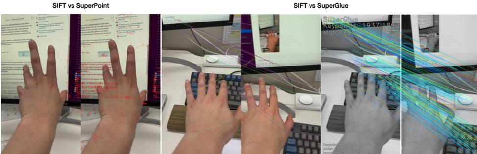
**Figure 3.4** Comparison of SIFT feature detection with SuperPoint on the left and SIFT feature matching with SuperGlue on the right. Results show that SuperPoint and SuperGlue show superior performance than SIFT in both feature detection and matching.
