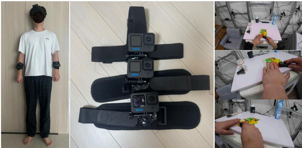
**Figure 3.1.** The setup of our system. The left section depicts the capture environment, the middle section highlights the GoPro cameras attached to their mounts, and the right section demonstrates a synchronized capture from all three cameras.
