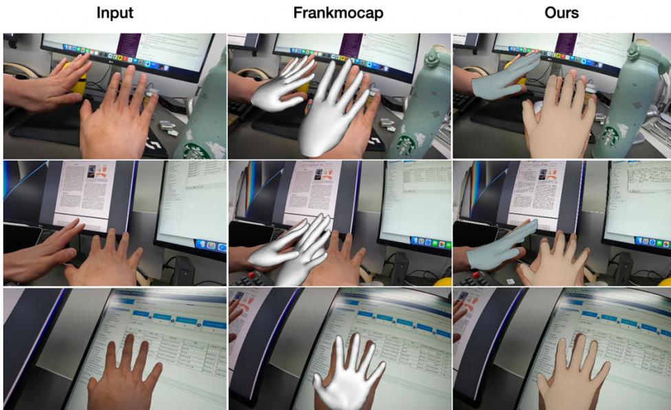
**Figure 4.3.** Qualitative comparison on our collected test set against Frankmocap. Our approach generally produces more plausible results and accurate hand orientations.
